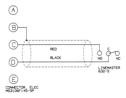
Figure 1.40071G-04Footswitch Assembly Schematic Diagram.
